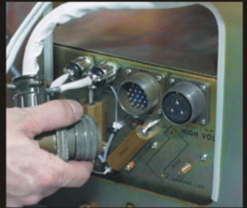
Repeat for second of two amphenol connectors.
