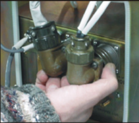
Unscrew first of two amphenol connectors.
