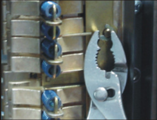
Spread circlip on end of pin open with regular pair of plyers.
