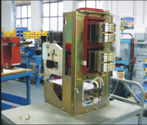
FBK circuit breaker with CP trip unit after replacement. Back view.
